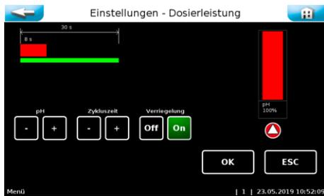
The picture below shows the Dosing performance menu when the control type 2-point or time control was selected for the disinfectant dosing.
