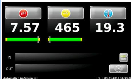
If one of the two measuring values, pH or mV, falls outside the control range, the start routine is activated.
