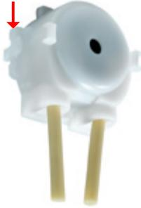
As part of the annual maintenance, the two dosing cartridges should be replaced. To do so, compress the two lateral expansion tabs and pull the head from the motor shaft toward the front. Unwind the two black cable ties from the hose end and pull the hoses from the hose nipples.
