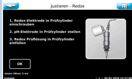
The Calibration → redox electrode menu enables a fine-tuning of the redox measurement. The redox test solution supplies a voltage of 468 mV at 25 °C, see bottle label.
