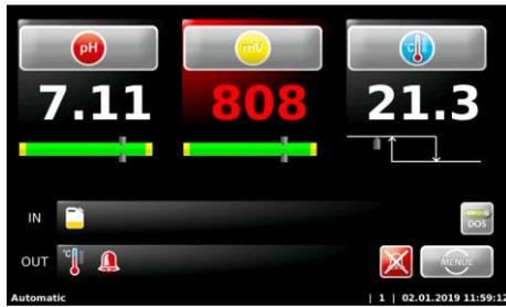
An alarm occurs; this is signalled by the
